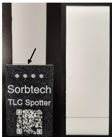
Figure 2 - Baseline is drawn at the top of the spotting guide where arrow is shown, the result is shown on the right.
