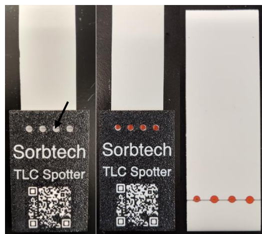
Figure 3 - When placed in the lower indent, the baseline will line up with the guide holes, sample is spotted through the holes, and the TLC plate is ready to run.
