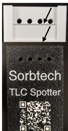
Figure 1 - The back of the guide (top photo) is indented with two steps as shown to allow for placement of the TLC plate for baseline drawing and spotting.
