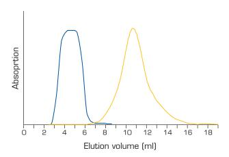
Elution profile overlay of 2.5 µmol 5-TAMRA and 0.25 µmol oligonucleotide (2.5 ml sample volume).
