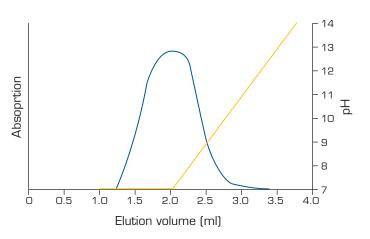
Separation of 10 M ammonia and oligonucleotide after cleavage from solid support and removal of protecting groups (18-mer, Scale:  $0.2~\mu mol$ , 1 ml sample volume). Elution with water.
