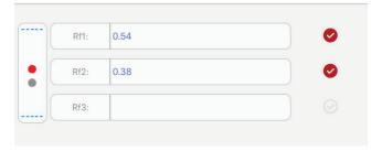
When any of the Rf values are selected, it is displayed as . If any of the Rf values are selected, then the software will generate a gradient curve automatically. If none of the Rf values are selected, then the gradient curve has to be adjusted manually. Click "next" to go to the next screen.
