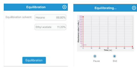
Click on "equilibration" when the ratio is set. It will open a pop-up window with the graph that shows absorbance of equilibration solvent. With this, users can pause or stop the equilibration manually. Otherwise, the system will decide the equilibration time based on the column size and stop automatically after that.
