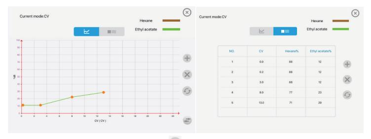
The gradient nodes can be added by clicking . The slope and duration of the gradient segment can be changed by clicking on the node and then dragging the node to a point of choice. The last created gradient segment can be deleted by clicking on . By clicking on the bottom right icon, users can toggle the unit of the x-axis between CV and minutes. Click on the top right icon exit the screen. Click "next" to go to the next screen.
